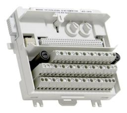
The TU839 MTU can have up to 8 I/O channels and two groups of connections for sensor power distribution. Each channel has two I/O connections. The process voltage can be connected to two individually isolated groups for sensor power distribution. Each group has a 200 mA fuse. The maximum rated voltage is 250 V and maximum rated current is 1 A per channel. It is recommended that the fuse rating be chosen to meet the applications needs.
