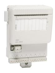
The Al801 Analog Input Module has 8 channels for current input. The current input is able to handle a short circuit to the transmitter supply at least 30 V d.c without damage.
