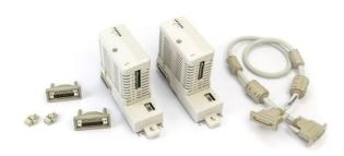
The BC810 unit consists of two basic parts: baseplate (TP857) and power supply/logic board. The baseplate is where the connectors to CEX-Bus and the external power reside. It is grounded to the DIN-rail through metal parts of the housing. The board also carries the external power voting diode and fuse. The power supply and logic board contain the +3.3 V converter, logic, drivers for CEX-Bus interconnection, and the connector for the interconnection cable.
