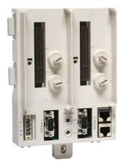
The TU846 is a module termination unit (MTU) for redundant configuration of the field communication interface Cl840/Cl840A and redundant I/O. The MTU is a passive unit having connections for power supply, two electrical ModuleBuses, two Cl840/Cl840A and two rotary switches for station address (0 to 99) settings.
