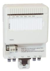
S800 I/O is a comprehensive, distributed and modular process I/O system that communicates with parent controllers and PLCs over industry-standard field buses. TB826 is a Long range Optical Media Converter for the ModuleBus. It is used to convert between plastic/opto fiber of HCS fiber with versatile link connectors and single mode field fiber with SC connector.
