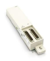
The TB846 redundant ModuleBus Cable Adaptor is used together with TB845 and two TK801V0xx to extend the ModuleBus. Using this extension I/O modules on the same electrical ModuleBus can be mounted on different DIN rails. TB846 can also be used together with TB842 to provide an optical extension of the ModuleBus.
