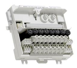
The TU837V1 MTU can have up to 8 I/O channels. The maximum rated voltage is 250 V and maximum rated current is 3 A per channel. The MTU distributes the ModuleBus to the I/O module and to the next MTU. It also generates the correct address to the I/O module by shifting the outgoing position signals to the next MTU.
