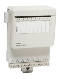
The DO802 is an 8 channel 110 V d.c./250 V a.c. relay (NO) output module for the S800 I/O. The maximum voltage range is 250 V and the maximum continuous output current is 2 A. All outputs are individually isolated. Each output channel consists of optical isolation barrier, output state indication LED, relay driver, relay and EMC protection components.
