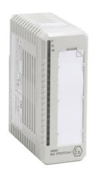
The AI893 Analog Input Module has 8 channels. The module includes Intrinsic Safety protection components on each channel for connection to process equipment in hazardous areas without the need for additional external devices.
