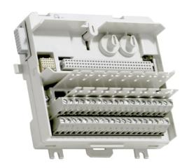
The TU834 MTU can have up to 8 I/O channels and 2+2 process voltage connections. Each channel has two I/O connections and one ZP connection. Input signals are connected via individual shunt sticks, TY801. The maximum rated voltage is 50 V and maximum rated current is 2 A per channel. The MTU distributes the ModuleBus to the next MTU. It also generates the correct address to the I/O modules by shifting the outgoing position signals to the next MTU.
