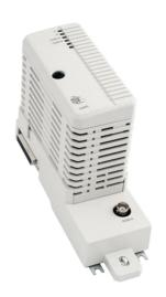
The CI865 module is the AC 800M system's communication interface for Satt ControlNet and bridges different bus standards used on AC 800M and Satt ControlNet. The CI865 module makes it possible to use older Satt I/O system (Rack I/O and Series 200 I/O) with the AC 800M controller platform, but it cannot be used as a general ControlNet interface. CI865 cannot be used in a High Integrity
