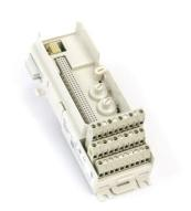
The TU811V1 is a 8 channel 250 V compact module termination unit (MTU) for the S800 I/O. The MTU is a passive unit used for connection of the field wiring to the I/O modules. It also contains a part of the ModuleBus.
