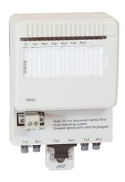
S800 I/O is a comprehensive, distributed and modular process I/O system that communicates with parent controllers and PLCs over industry-standard field buses. TB826 is a Long range Optical Media Converter for the ModuleBus. It is used to convert between plastic/opto fiber of HCS fiber with versatile link connectors and single mode field fiber with SC connector.
