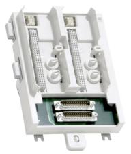
The TU852 is a 16 channel module termination unit (MTU) for redundant S800 I/O modules and for mounting on a horizontal DIN rail. The MTU is a passive unit used for connection of the field wiring to the I/O modules. It also contains a part of the ModuleBus.
