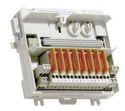
The TU835V1 MTU can have up to 8 I/O channels. The maximum rated voltage is 50V and maximum rated current is 2 A per channel. The MTU distributes the ModuleBus to the I/O module and to the next MTU. It also generates the correct address to the I/O module by shifting the outgoing position signals to the next MTU.
